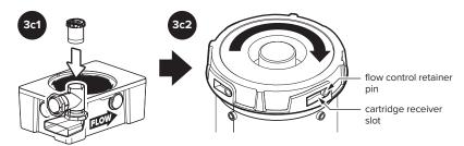
Slide flow control cartridge into top of inlet diffuser and rotate clockwise until cartridge drops onto flow control retainer pins. Continue rotating clockwise until pins are fully seated.
