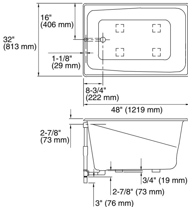
No change in measurement if connected with drain illustrated. (K-7163)
