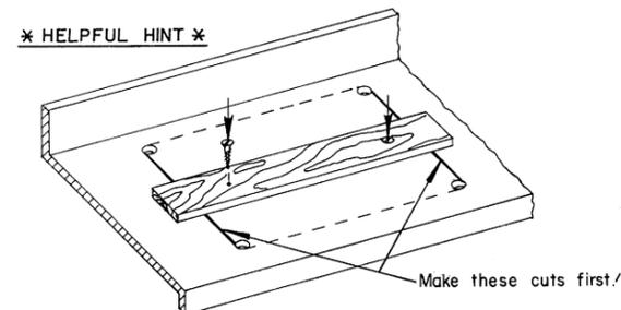
After making cuts along sides of cutout, secure a board as shown to prevent cutout from possibly damaging countertop or prematurely dropping.
