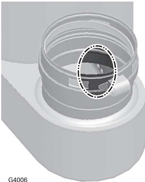
Figure 79 Recuperator flueway drain holes
