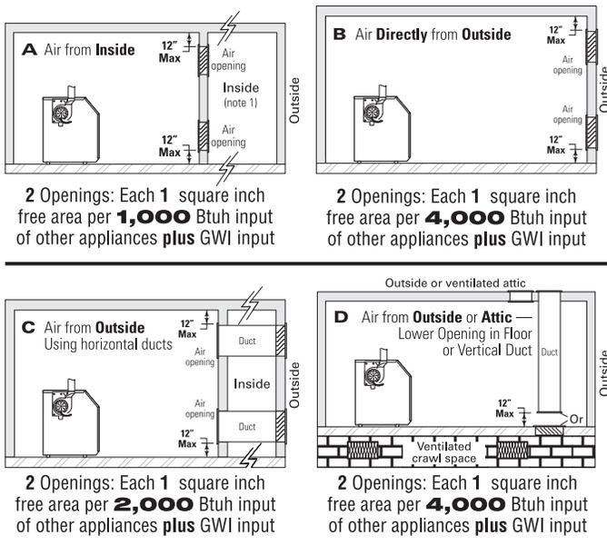
**EXCEPTION: NO** combustion air openings are needed when the boiler (and other appliances) are installed in a space with a volume **NO LESS** than 50 cubic feet per 1,000 Btuh of all installed appliances. Sum the total input of all appliances in MBH (1,000's of Btuh) and multiply this number times 50. **Building must not be of Tight construction** (see definition below).
