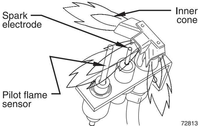
4. Incorrectly heated pilot flame sensor.
