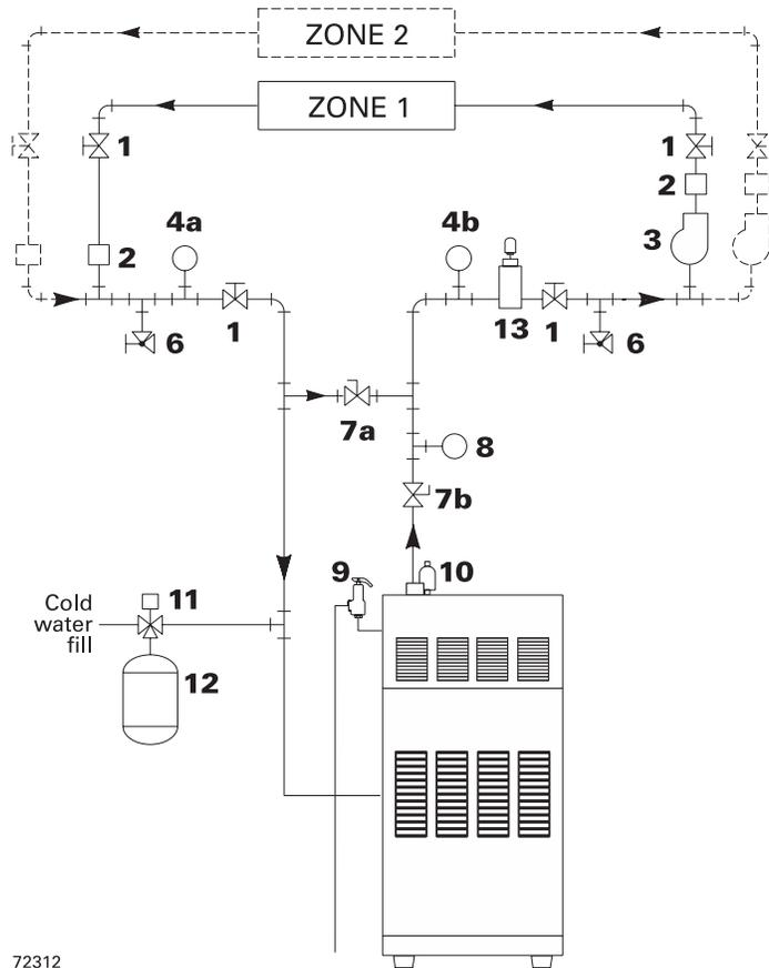
**Figure 19** Boiler-bypass piping
