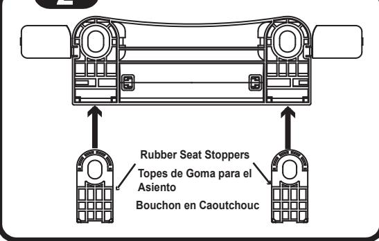
Add anti-skid, Rubber Seat Stoppers (A) to the corresponding grooves on the bottom of the Hinge Case. Make sure the Rubber Seat Stoppers lie flat against the Hinge Case.
