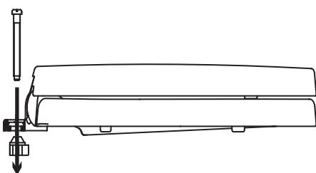
Insert Plastic Bolt (B) and tighten Plastic Nut (C) on underside of toilet.
