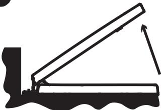
Flatten the Hinge Case against the toilet by holding the seat down and raising the lid. Hold the Hinge Case against the toilet and lower the lid.
