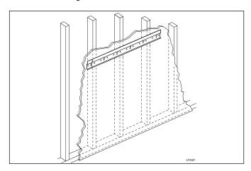
If only two screws can be used, install cross blocking (2" x 6") between the studs and then attach the wall mounting plate. Again, for double sinks install cross blocking (2" x 6") between the studs to add extra support for the wall mounting plate and the sink.
