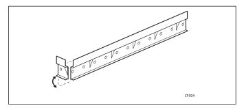
Position the top lip of the wall mounting plate on the mark. Be sure you mark the mounting holes over the studs/cross-blocks. Use a bubble level to make sure the wall mounting bracket is level.
