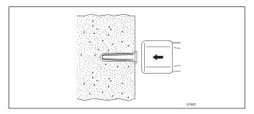
Attach the mounting plate to the wall with 1/4" x 1-1/2" long Phillips head screws (supplied with unit). For single bowl models use at least three screws. For double bowl models use at least six screws.
