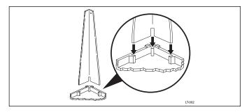
3. Place a block of scrap wood over the end of the leg and drive the leg down into the socket with a hammer.
