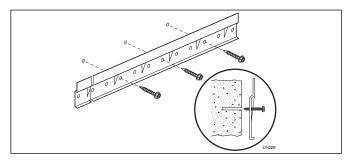
**Note:** Make sure the wall mounting plate is straight, regardless of the wall contour, before completely tightening the screws. If wall is not flat, shim behind the mounting plate, as needed.
