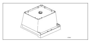
Slide the metal or plastic leg into one of the plastic corner retaining sockets in the bottom of the laundry tub. All four legs are identical and can be installed in any one of the four corners.
