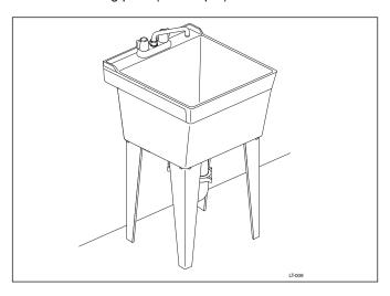
On wall mount models only, lift and place the sink over the wall mounting plate. Make sure the laundry tub is seated securely into the lip of the wall mounting plate.
