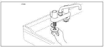
**Note:** Preinstallation of the faucet, supply lines, and P-trap are easier when the laundry tub is not against and/or attached to the wall.
