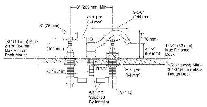
Rim or Deck-Mount Installation Rough + Finished Deck-Mount Installation
