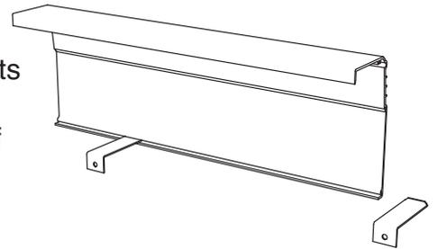
6. Position new assembled cover with wall brackets below element, then slip new cover over back panel.
