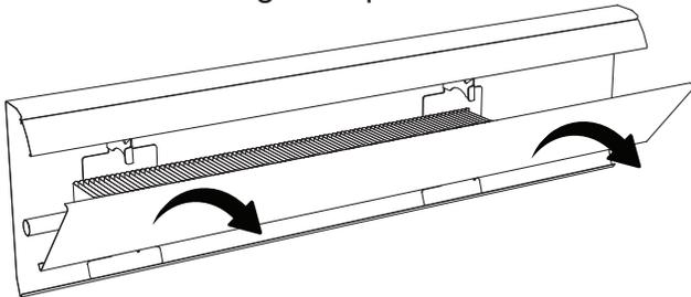
3. Remove any existing damper sections.
