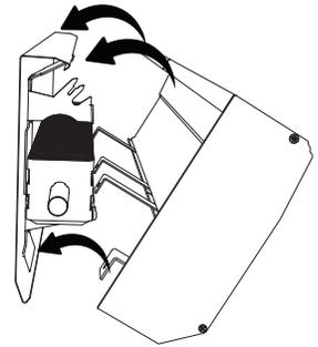
7. *Optional:* Screw brackets to existing back panel with supplied self-drilling screws.
