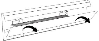
3. Remove any existing damper sections.
