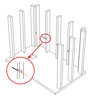
6. Install tub and mark top of tile flange with pen
