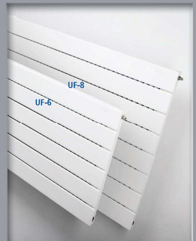
Runtal offers 2 wall panels (6 and 8 panels) in 2', 3', 4' and 6' lengths in stock in white for immediate delivery. All stock wall panels have multiple tappings (AB) that allow for all types of bottom and side piping connections (See piping configuration AB on page 13, Table 3). Stock wall panels may be special ordered in any of the other nine standard colors with a two-week delivery.
