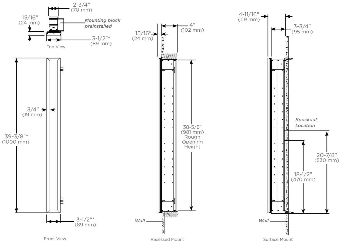
\*Lens dimensions are 1/8" (3 mm) smaller than light body
