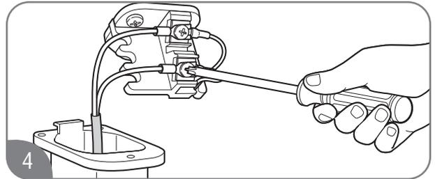
4 Firmly tighten the terminal screws by hand.
