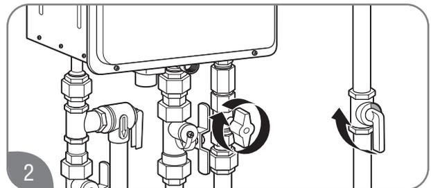
Close the gas shut-off valve(s).
