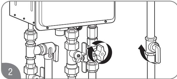
2 Close the gas shut-off valve(s).
