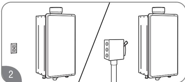
Make sure the proper electrical outlet or supply (120 VAC/60 Hz) is available and located near the unit. Direct-vent models come with a 6-ft. (1.8-m) power cord, while the outdoor models require hard-wiring or the addition of a plug.
