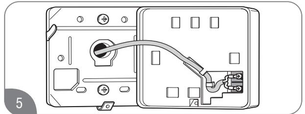
Connect the remote control to the remote control cable.
