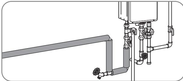
Long hot water lines should be insulated to conserve water and energy.
