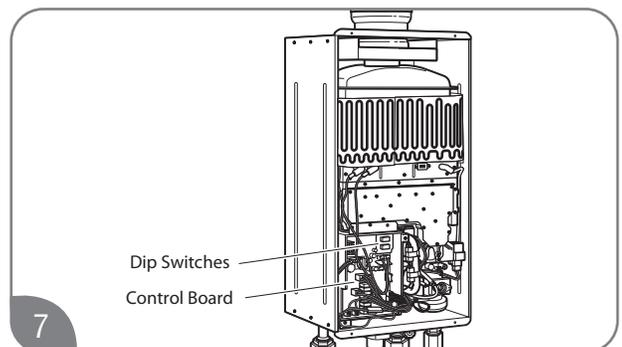
7 Find DIP Switch 2 in the top-right portion of the control board. The switch labeled "DIP 2" is the bottom switch.
