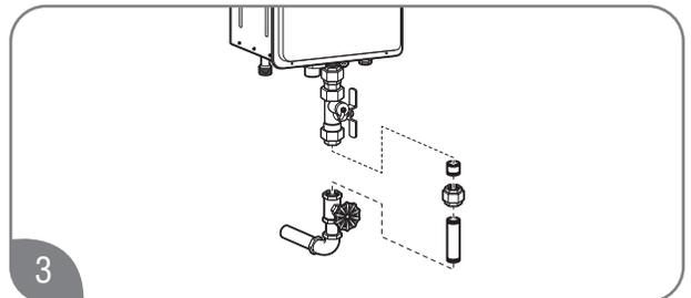
Install a service valve on the end of the COLD water supply line and connect it to the water inlet on the water heater.
