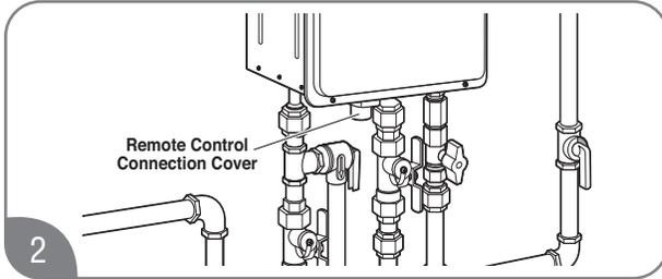
2 Loosen the one screw located on the remote control connection cover. The connection cover is made of white plastic.
