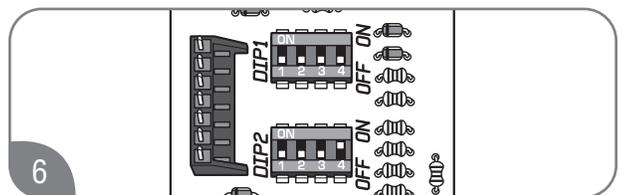
6 If altitude is above 5,400 ft. (1650 m) and below 8,500 ft. (2590 m), change the fourth switch to the ON position (UP).
