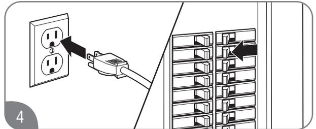
4 Turn on all electric power to the water heater. The water heater burner will automatically light when there is a demand for hot water.
