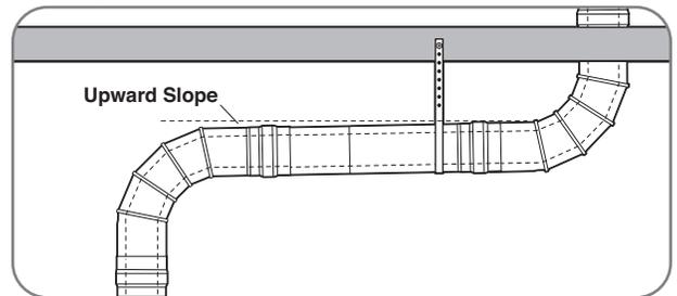
When a water heater is vented vertically, an UPWARD slope must always be used. Always attach a drain hose to the condensate collector and plumb the hose to a sanitary sewer drain.
