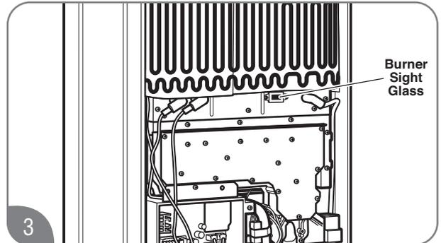
While the water heater is operating, inspect the main burner flames through the burner sight glass. The flames should be blue when the main burner is firing.
