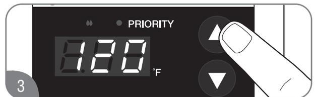
Press the UP adjustment button repeatedly until 120°F (49°C) shows in the LED display. Hold the UP button until “140” on the display starts to blink.
