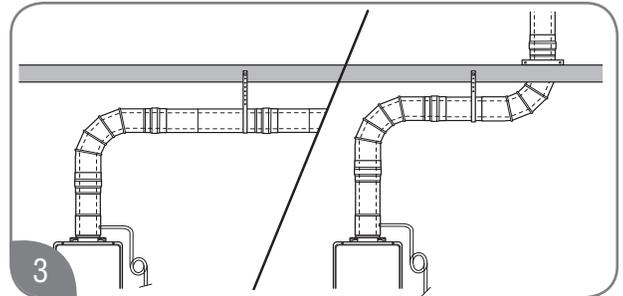
Support vertical and horizontal runs as described on "Venting". Vertical supports are required every 4 ft. (1.2 m) along a vertical pipe route, after every transition to vertical, and after every offset elbow.
