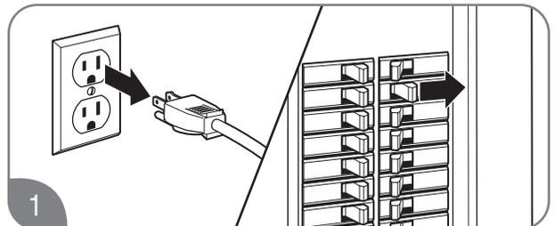
1 Disconnect all electric power to the water heater.
