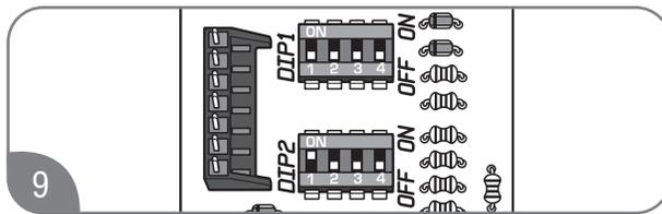
9 Change the first switch on “DIP 2” to the ON position (UP). Performance mode is selected.
