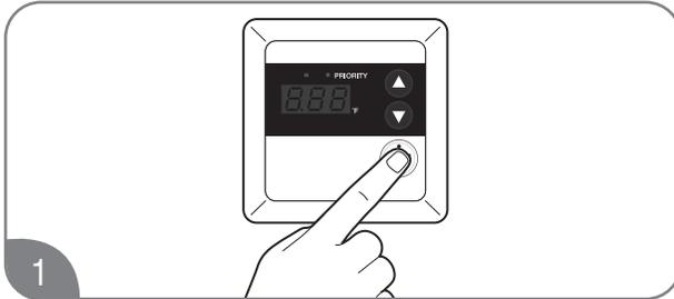
1 Turn off the water heater by pressing the POWER ON/OFF button on the control panel.
