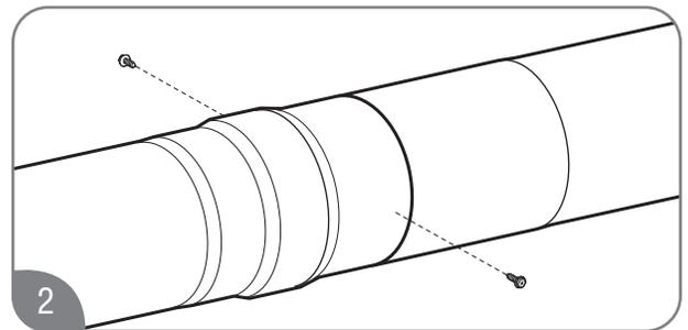
Attach the female end of the next vent pipe section to the male end of the 3-in./5-in. (7.6-cm/12.7-cm) concentric vent pipe. Push firmly on the pipe until the outer jacket has made contact with the snap ring on the male end of the concentric vent pipe section. Secure the two pipe sections with the provided self-tapping screws.
