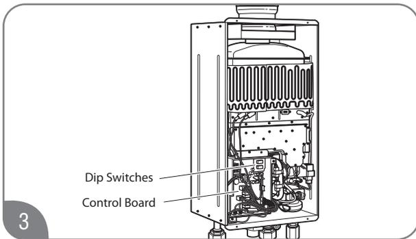
Find DIP Switch 1 located in the top-right portion at the control board. The switch labeled “DIP 1” is the top switch.
