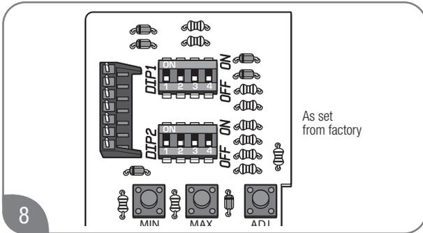
8 The factory setting for this switch should all be in the OFF position (DOWN).
