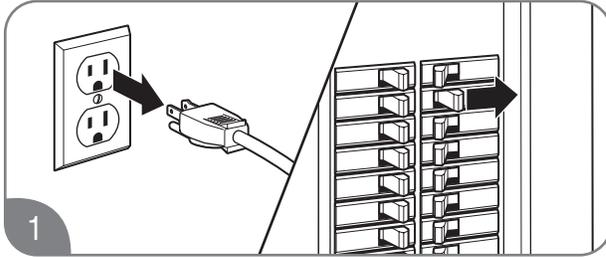
1 Ensure that the power to the water heater has been disconnected.
