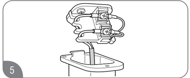
5 Secure the remote control extension cable on the hook located on the side of the remote control connection base.
