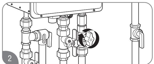
2 Turn the gas shut-off valve clockwise to the OFF position.
