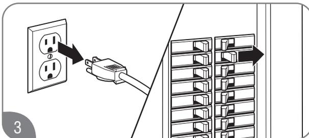
3 At least 10 seconds after Step 1, unplug the water heater or disconnect the power supply at the circuit breaker box.
