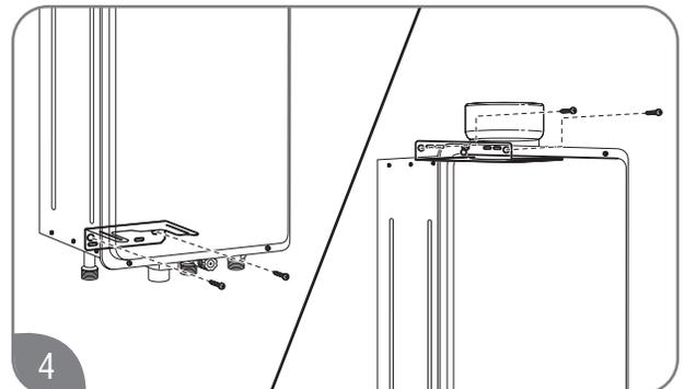
Using two mounting screws and washers, secure the lower mounting bracket to the wall. Then, secure the upper mounting bracket to the wall with two mounting screws and washers.
