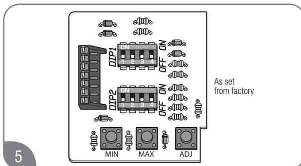
The factory settings for this switch should all be in the OFF position (DOWN).
