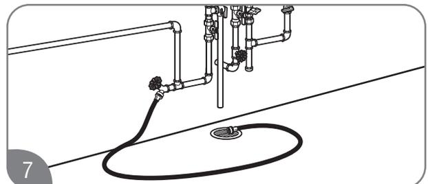
7 Connect a garden hose to the drain valve in the hot water outlet line and place the other end in a suitable drain. Open the drain valve until all the water has drained from the water heater. Leave water heater as is until placed back in service.
