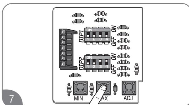
Push and hold "Max" button until "ON" is shown on the display of the remote control.
