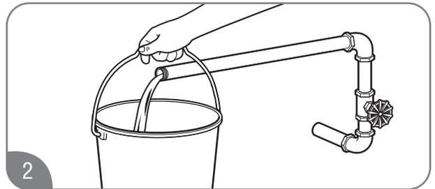
Before attaching the water line to the water heater, open the shut-off valve. Run the water until it has purged all contaminants (sand, debris, air, caulking).
