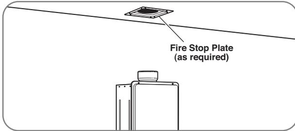
Every vent pipe penetration of a floor or ceiling that is not in a fire-rated shaft requires a fire stop plate.
