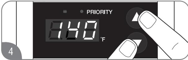
4 While "140" is blinking, press the UP and DOWN adjustment buttons at the same time. "140" will appear without blinking.
