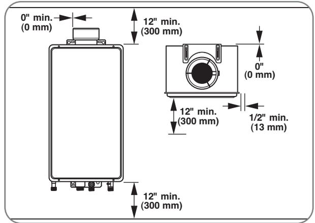
Minimum water heater clearances from combustible and noncombustible construction are as follows:
