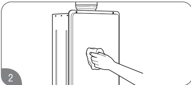
Clean the water heater and the remote control with a damp soft cloth and mild detergent. Gently wipe and completely dry all surfaces.
