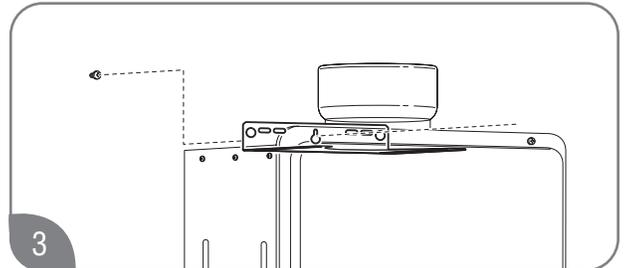
Position the upper mounting bracket and partially install the center mounting screw. The clearance between the screw head and the wall should be about 1/8 in. (0.3 cm). Hang the upper bracket on the screw.
