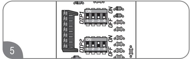
5 If altitude is above 2000 ft. (610 m) and below 5,400 ft. (1650 m), change the third switch on "DIP 2" to the ON position (UP).
