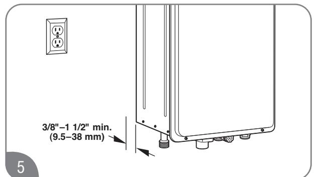
Position the water heater and tighten the adjustment screws to complete the installation. The rear of the water heater can be positioned anywhere between 3/8 in. (0.95 cm) and 1 1/2 in. (3.8 cm) from the wall (indoor model only).
