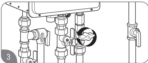
3 Turn the gas shut-off valve counterclockwise to the ON position.
