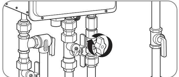
The water heater and its manual gas shut-off valve must be disconnected from the gas supply piping system whenever the pressure testing will exceed 1/2 psi (14 in. w.c. [3.5 kPa]).
