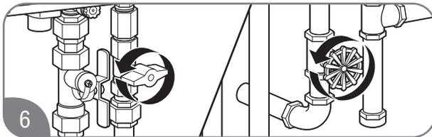
6 Turn on the gas and water to the water heater by opening the shut-off valves.
