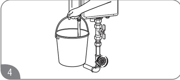
Open the drain valve in the COLD water outlet line to check the water flow through the water heater.
