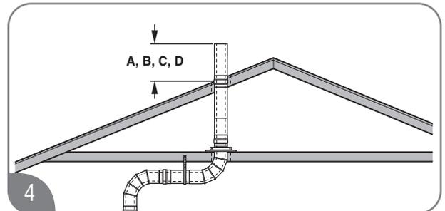
Determine the vent terminal height and install the vent pipe accordingly. Refer to "Vertical Vent Terminal Location" on this Use and Care Manual for clearance requirements.
