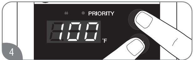
Press and hold the DOWN and UP adjustment button for 5 to 10 seconds.
