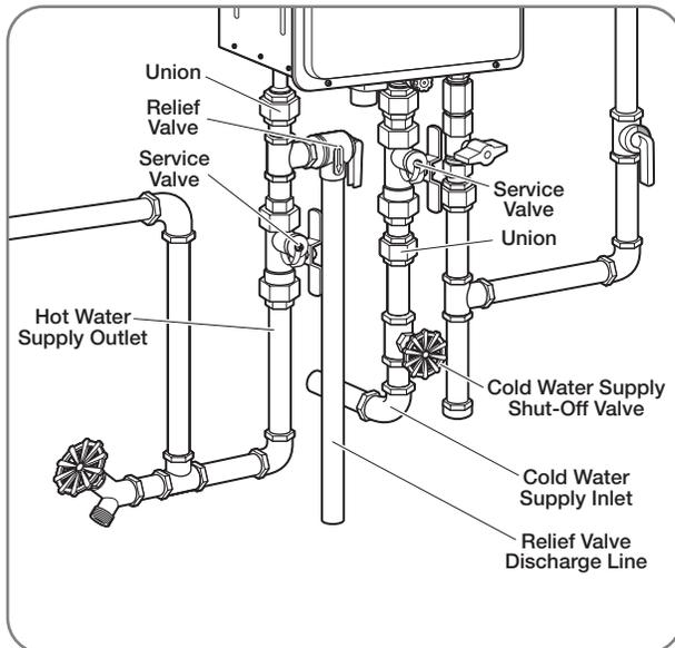
One end of the relief valve discharge line connects to the HOT water outlet pipe as shown above. The other end of the pipe should be routed to a suitable drain to eliminate potential water damage.
