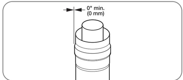
Minimum clearance around the coaxial vent pipe should meet the specifications listed on the instruction/warning label on the water heater. If no label is found, use the vent manufacturer's specifications or a minimum clearance of 0 in. (0 cm) around the vent pipe.
