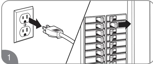
1 Disconnect all electric power to the water heater.
