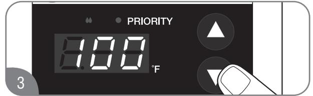
Press the DOWN adjustment button repeatedly until 100°F (38°C) shows in the LED display.
