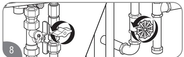
8 Turn on the gas and water to the water heater by opening the shut-off valves.
