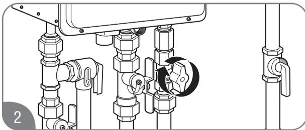
2 Turn the gas shut-off valve clockwise to the OFF position. This valve is located on the outside of the water heater. Wait 5 minutes to clear any gas. If you don't smell gas, proceed to Step 3.
