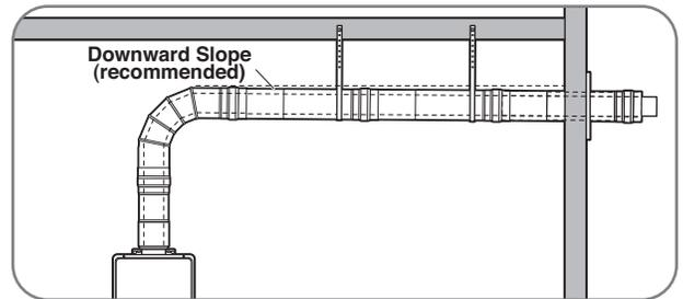
When a water heater is vented horizontally, the vent pipe should have a DOWNWARD or UPWARD slope towards the termination. If an UPWARD slope is used, always attach a drain hose to the condensate collector and plumb the hose to a sanitary sewer drain.
