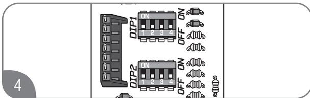
Change the third switch on “DIP 1” to the OFF position (DOWN).
