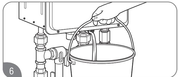
6 Using a suitable container to catch the water, remove the water filter from the base of the cold water inlet line.
