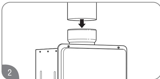
Complete the vent pipe installation to the water heater vent collar. If required, use high temperature silicone sealant where the vent connector joins the water heater.
