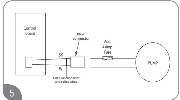
5 To connect to the pump, cut the blue connector, splice the wires, and add a 4 amp fuse to the hot wire of the pump.
