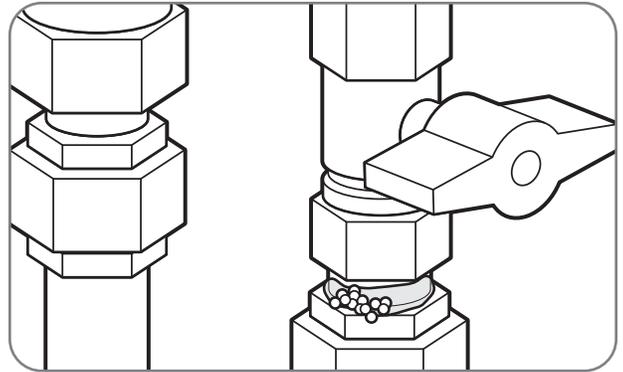
Turn on the gas shut-off valve(s) to the water heater.
