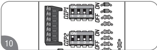
10 To select Energy Saver mode, change the fourth switch on “DIP 1” to the ON position (UP).
