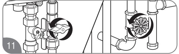
Turn on the gas and water to the water heater by opening the shut off valves.
