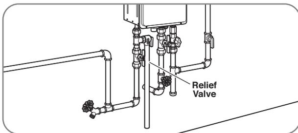
Annually check the operation of the pressure-relief valve. Lifting the lever handle on the pressure-relief valve opens the valve to flush hot water through the discharge line to the drain. After several gallons have drained, release the lever handle to close the valve and stop draining.
