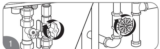
Turn off the gas and water to the water heater by closing the shut-off valves.
