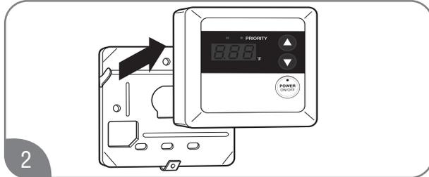
Remove the remote control from the base plate.
