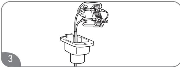
3 Connect the remote control extension cables from the remote control to the remote control connection terminals.
