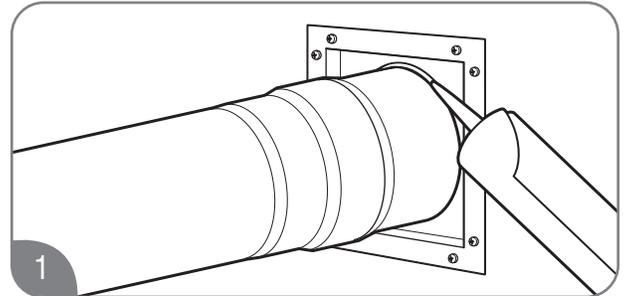
Apply high temperature silicone sealant or silicone/latex caulk around the vent section. Completely seal where it passes through the wall plate and where it is attached to the structure. This will provide a weather seal for the system, so it must be a good seal.
