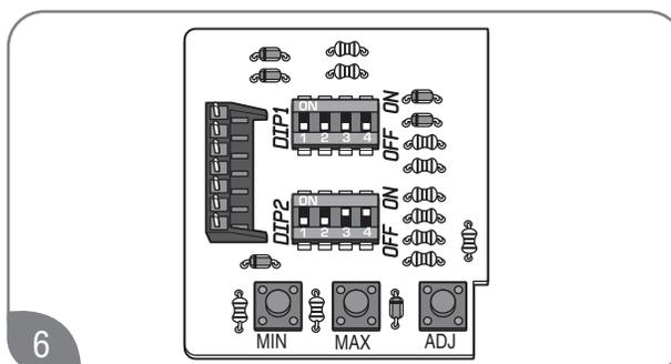
Change the third and fourth switches on "DIP 2" to the ON position (UP).
