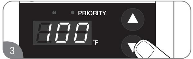
3 Press the DOWN adjustment button repeatedly until 100°F (38°C) or 85°F (29°C) shows in the LED display. Hold the DOWN button until the number on the display starts to blink.
