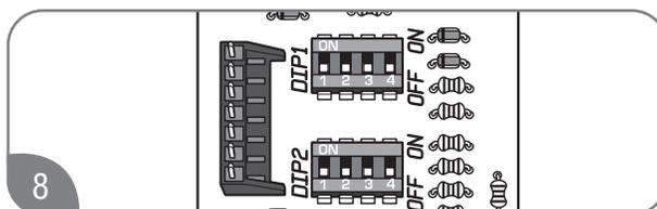
Change the third and fourth switches on "DIP 2" to the OFF position (OFF).
