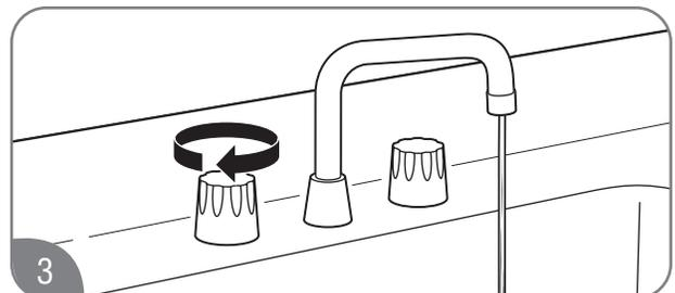
Open a hot water faucet slightly until the water stream is approximately 1/8 in. (0.3 cm). Be sure to check the flow periodically.
