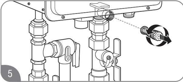
Close the shut-off valve and remove, clean, and replace the water filter.
