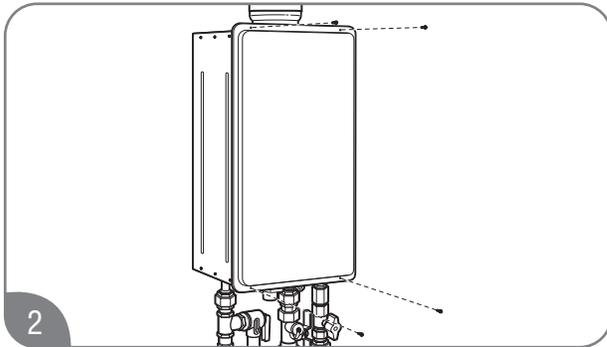
Remove the front cover panel on the water heater.
