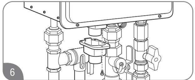
6 Reinstall the remote control connection cover and secure with the one screw.
