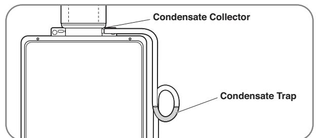
The drain tube is fashioned into a "pigtail" trap and must be filled with water to prevent flue gases from emitting into the building prior to operating the water heater.
