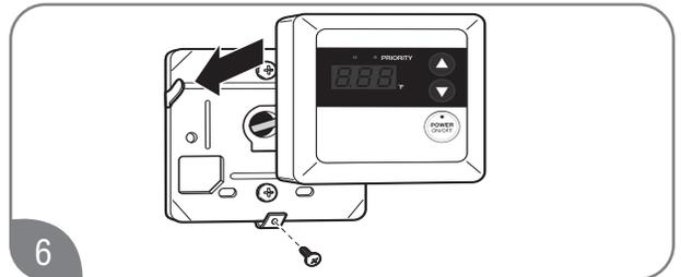
Position the remote control on the base plate.
