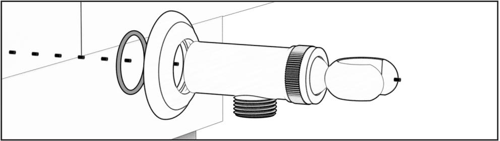
Slide Flange against the wall. **NOTE: the hook is tapered to accept the cone fitting of hand shower hose. If the hose will not slide into the hook, rotate the hook assembly 180°.**
