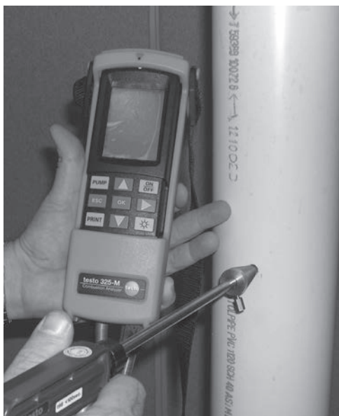
Figure 9.2: Insert Analyzer Test Probe into Test Port
