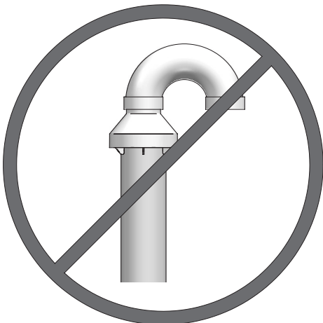
Figure 5-5 Do Not Install U-Bend to Rain Cap
