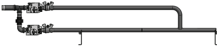
Figure 8-5 _Gas Train 500,000 Btu/hr Model
