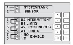
Figure 5-5\_Remote on/off boiler
