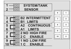
Figure 5-4\_Stand-alone operation water heater
