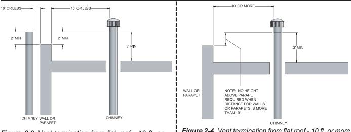
**Figure 2-3\_**Vent termination from flat roof - 10 ft. or less from parapet wall
