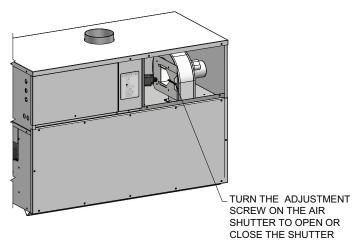
**Figure 8-4**\_Combustion air adjustment with manometer to set differential pressures
