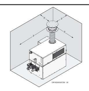
Figure 2-8\_Outdoor vent kit installed on Models 497 - 747
