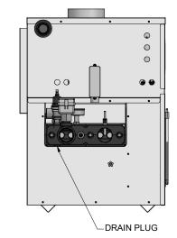
Figure 1-2B\_Drain the unit\_Models 987 - 2067
