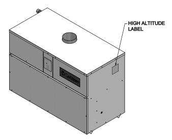
Figure A High altitude label location\_boiler
