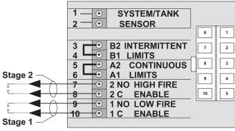
Figure 5-8\_Field installation safety devices
