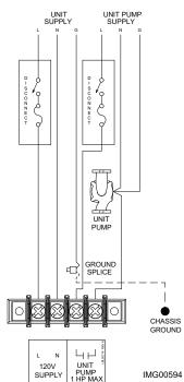
Figure 5-2\_Line Voltage Field Wiring Connections
