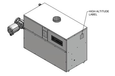
Figure B High altitude label location\_water heater
