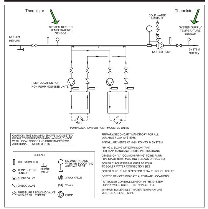
Figure 11. Hydronic Piping - Primary-Secondary, Reverse-Return.
