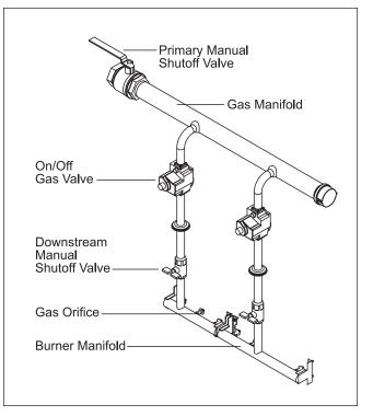
Figure 46. Typical Gas Train Configuration.
