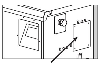
Figure 22. Access Panel for Field Connections
