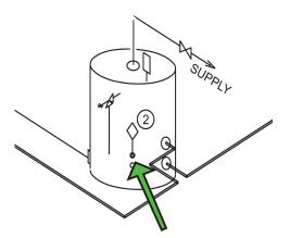
Figure 7. Location of DHW Tank Sensor
