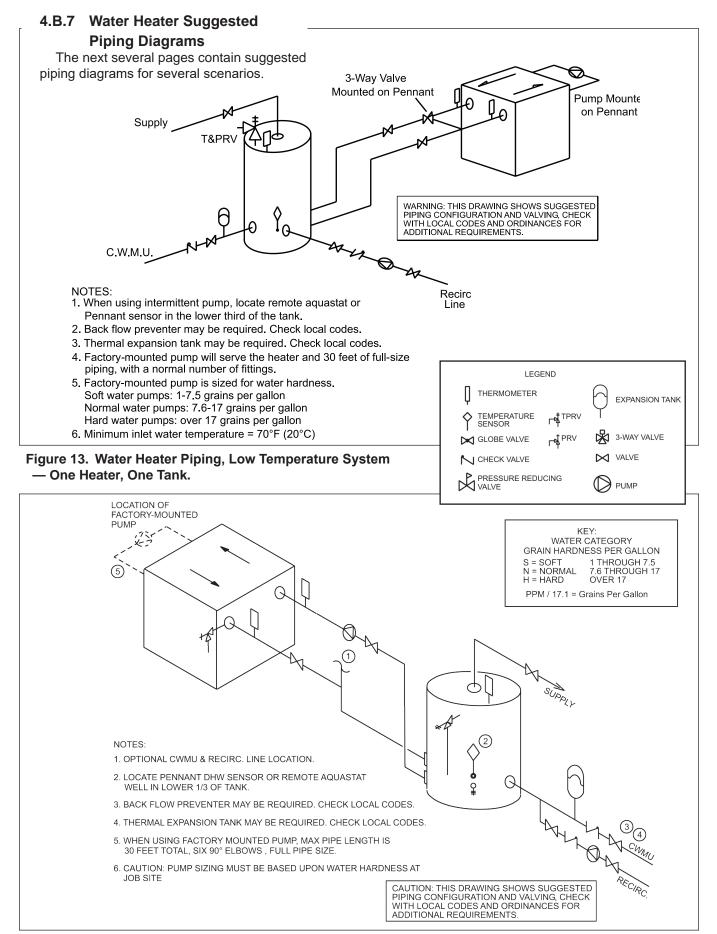
Figure 14. Water Heater Piping— One Heater, One Tank.
