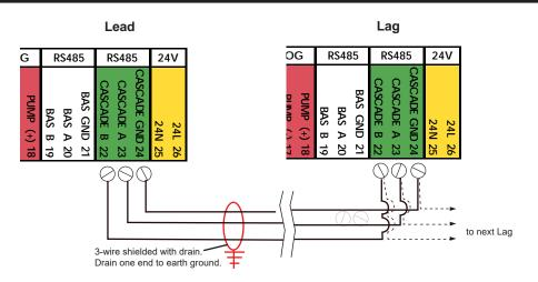
Figure 25. Cascade Wiring Connections
