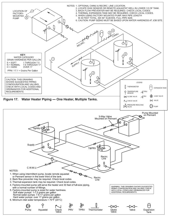
Figure 18. Suggested Piping, Low Temp System — One Water Heater, Multiple Tanks.
