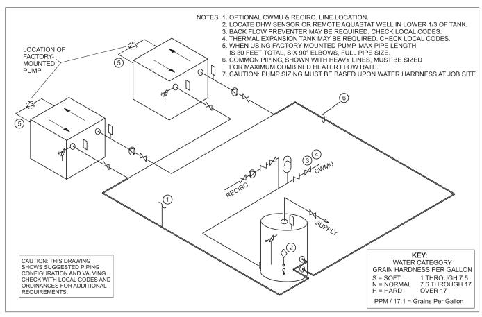
Figure 15. Water Heater Piping — Multiple Heaters, One Tank.
