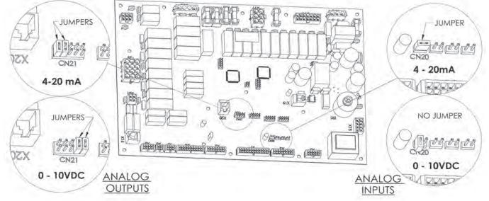
Figure 23. Analog Input and Output Jumper Placement
