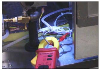
Figure 42. Amp Meter looped around an HSI wire.
