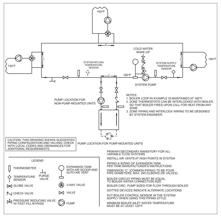
Figure 8. Hydronic Piping — One Boiler, Multi-Temperature System.
