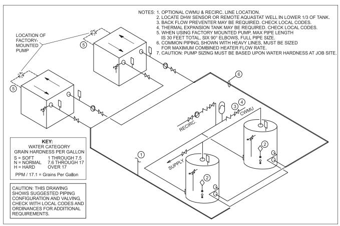
Figure 19. Water Heater Piping — Multiple Heaters, Multiple Tanks.
