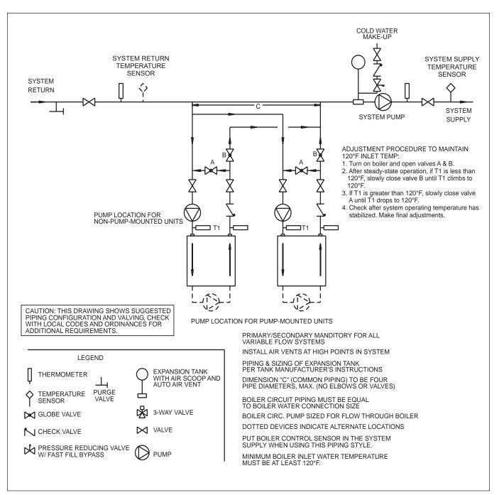
Figure 12. Hydronic Piping - Primary-Secondary, Reverse-Return, Low Temperature.
