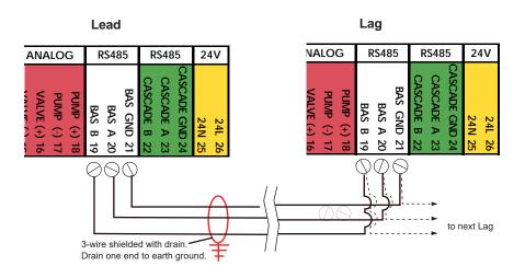
Figure 26. BMS Wiring Connections
