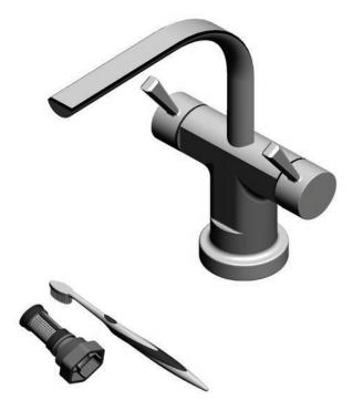
8. To refill the combination boiler, reassemble the filters back into the combination boiler and reverse steps 6 back to 1.
