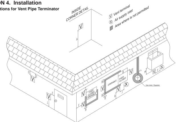
\* For clearances not specified in ANSI Z224.1 / NFPA 54 or CAN/CSA-B 149.1, please use clearances in accordance with local installation codes and the requirement of the gas supplier.
