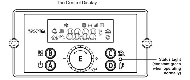
**The Control Display** has a Control Dial (E), 4 buttons (A, B, C, D), and a Liquid Crystal Display (with 72 back-lit segments). This section of this manual gives instruction on how to navigate into the many functions of the Mascot FT and to change temperature set points, set system variables and controller parameters.
