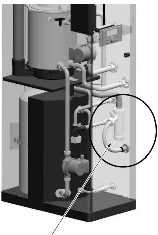
Condensate Trap and Drain Pipe (viewed from left front corner and as if the side and front panel are semi-transparent).
