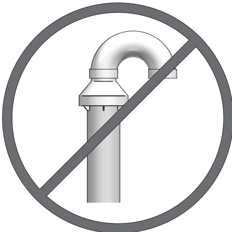
Figure 5-5 Do Not Install U-Bend to Rain Cap
