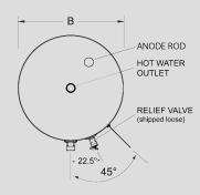
The "Hot Water Outlet" connection is Female NPT. All other connections are Male NPT.
