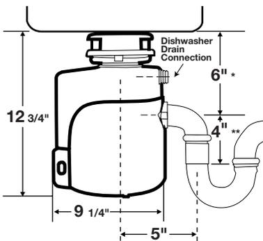
\*Distance from bottom of sink to center line of disposer outlet. Add 1/2" when stainless steel sinks are used.
