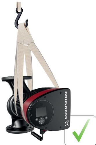
*Correct lifting of the pump*
