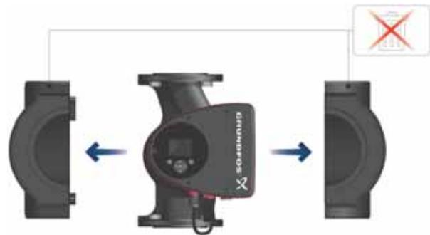
Fig. 3 Fitting insulating shells to the pump
