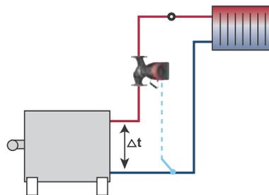
Fig. 27 Differential temperature
