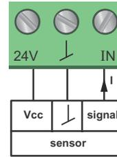
**Fig. 16** Analog input for external sensor, 4-20 mA
