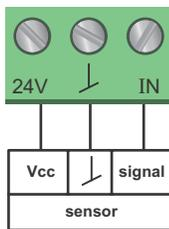
**Fig. 15** Analog input for external sensor, 0-10 V
