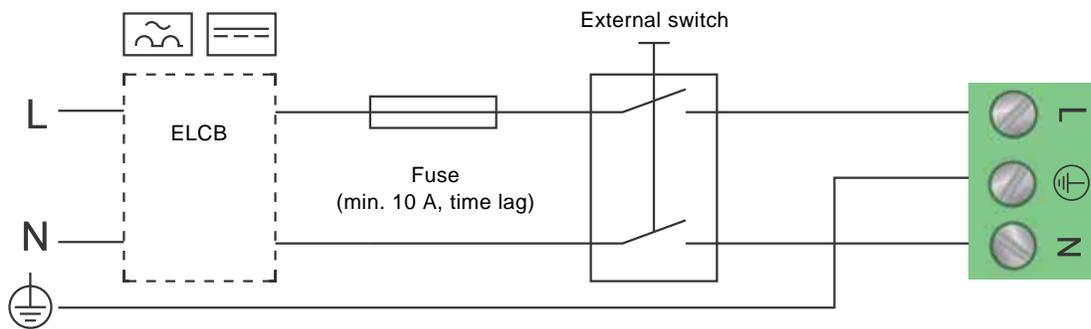
Fig. 11 Example of typical connection, 1 x 230 V ± 10 %, 50/60 Hz
