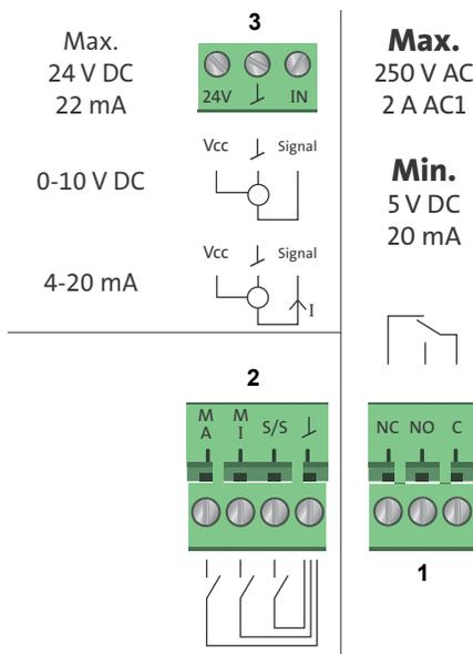
Fig. 12 Connection diagram
