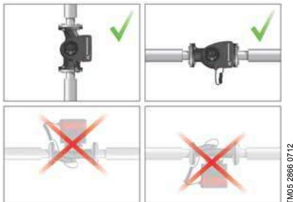
Fig. 35 Installation positions
