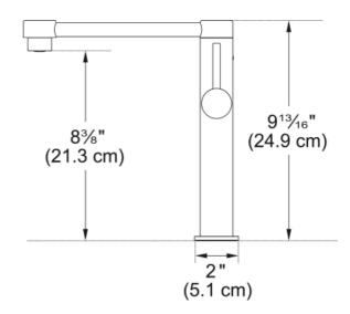
Pescara Polished Chrome 9.8-in Single Handle Swivel Spout Kitchen Prep Faucet. Pescara's solid brass construction ensures long- lasting performance. The ECO cartridge's built-in water saving feature helps conserve water during everyday kitchen tasks. The single handle effortlessly controls water temperature and pressure. ADA compliant
