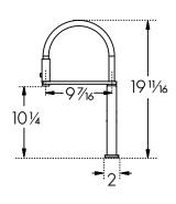
Faucet supply lines are U.S. standard 3/4" O.D. All faucets can accommodate at least 13/4" countertop thickness. Several can accommodate up to 3". Call for additional thickness.
