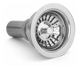
3 1/2" (89 mm) Type 316 (EN1.4401-17/12/2) stainless pull up crumb cup strainer with 1-1/2" x 3" (38 mm x 76 mm) Type 316 (EN1.4401- 17/12/2) stainless steel tailpiece, for enhanced corrosion resistance. Certified to ASME A112.18.2-2005/CSA B125.2-2005
