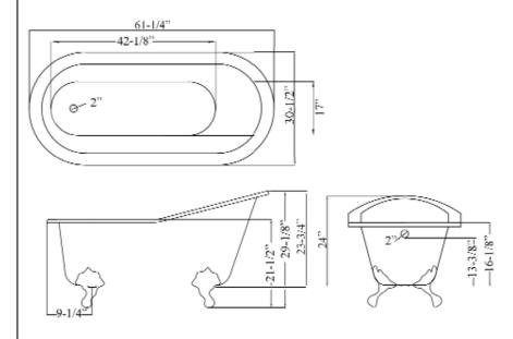
Dimensions of fixture are nominal and may vary within the range of tolerances established by ANSI Standard A112.19.1M. Dimensions and specifications subject to change without notice.
