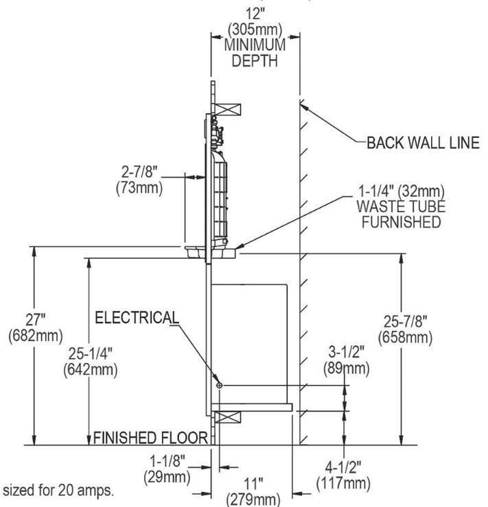
Note : New Installations Must Use Ground Fault Circuit Interrupter (GFCI). It is highly recommended that the circuit be dedicated and the load protection be sized for 20 amps.
