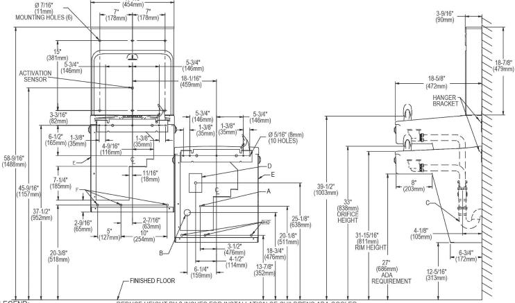
REDUCE HEIGHT BY 3 INCHES FOR INSTALLATION OF CHILDRENS ADA COOLER A = Recommended Water Supply location. Shut-off Valve (not furnished) to accept 3/8" O.D. unplated copper tube. Up to 3" (76mm) maximum out from wall. B = Recommended Waste Outlet location. To accommodate 1-1/2" nominal drain. Drain stub 2" (51mm) out from wall.
