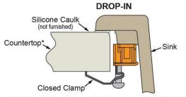
\*Maximum thickness for use of hold down system is 1-3/4" (44mm).
