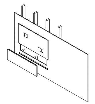
Includes the access panel and L-bracket for mounting. The access panel has a tab along the top which secures behind the fountain back panel. L-bracket is mounted to the wall. Access panel is secured to L-bracket with screws.
