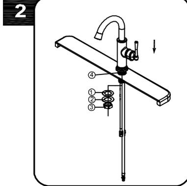
Place faucet through the hole in top of sink. From underside, assemble rubber washer ①, metal washer ② and nut ③ onto long shank ④ and tighten nut ③. Firmly tighten the nut ③ to metal washer ②. Do not overtighten.
