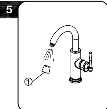
Important: after installation is completed, turn on hot and cold water supplies. Remove aerator ①. Turn faucet handle to the warm position where it mixes hot and cold water. Flush water lines for one minute. Check for leaks. Retighten any connections if necessary. Reinstall the aerator tightly.
