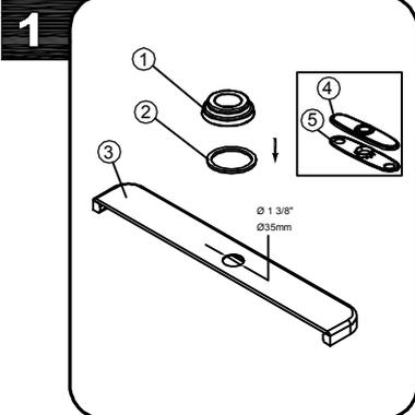
Shut off water supplies. Clean sink surface. Place washer ② and flange ① on the sink ③. If you do not use flange, please use escutcheon ④ and gasket ⑤ to replace flange and washer.
