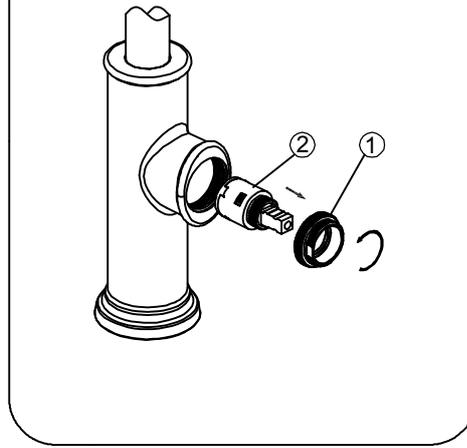
Loosen cartridge nut ① by turning it counter-clockwise and lift out the cartridge ②. Remove old cartridge and replace with new cartridge. Reinstall the handle.
