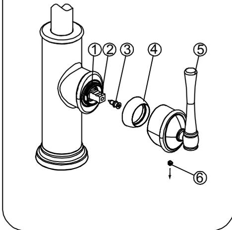
Shut off water supply! .With valves in "closed" position, unscrew set screw ⑥ and remove handle ⑤ from valve stem ②. Loosen the screw ③ from valve stem ②. Loosen the cap ④ from the cartridge nut ①.
