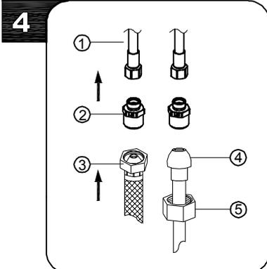
Make connections to water lines with 3/8" female compression supply hoses ①.
