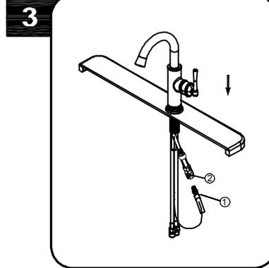
From underneath the sink, align block ① and tabs ② on quick connects. Push quick connect housing firmly upward and snap onto receiving block. Pull down moderately to ensure connection has been made. If it is necessary to remove quick connect, squeeze tabs on hose between index finger and thumb, then pull down to disconnect.
