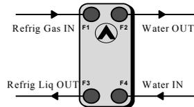
Fig. 4 Connection location: Condenser
