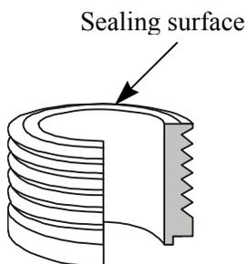
Some connections have an external heel. The purpose of the heel is to simplify the pressure and leakage testing of the BPHE in production.
