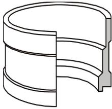
The soldering connections (sweat connections) are in principle designed for pipes with dimensions in mm or inches. The measurements correspond to the internal diameter of the connections. Some of DHT's soldering connections are universal, i.e. fit both the mm and inch pipes. These are denominated xxU, such as the 28U which fits both the 1 1/8" and 28.75 mm.
