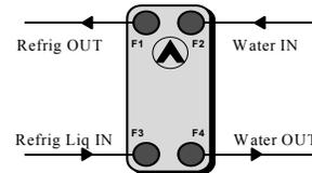
Fig. 5 Connection location: Evaporator
