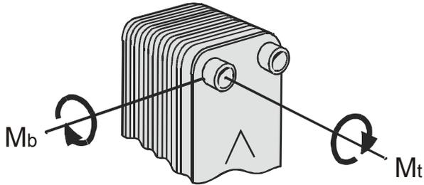
The maximum allowable connection loads given below are valid for low-cycle fatigue. The maximum allowable connection loads given below are valid for low cycle fatigue. If high cycle fatigue is involved special analysis should be made
