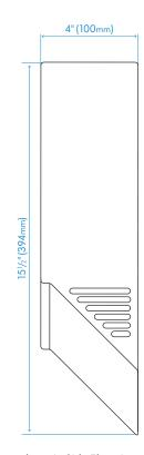
Machine fascia shown above in Side Elevation.
