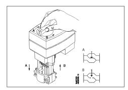
The manual override is achieved by turning the manual knob to the required position.
