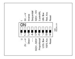
The actuator has a function selection DIP switch under the removable cover. In particular, if SW6 is set to ON, the actuator will perform as 3-point
