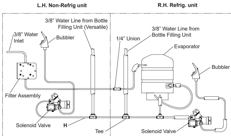
**EZ Bi-Level Plumbing Diagram after Filter Installation & Bottle
