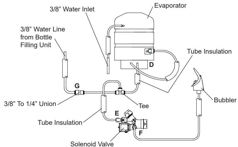
**EZ Plumbing Diagram after Pressurization Modifications****Fig. 7****L.H. Non-Refrig unit****R.H. Refrig. unit**
