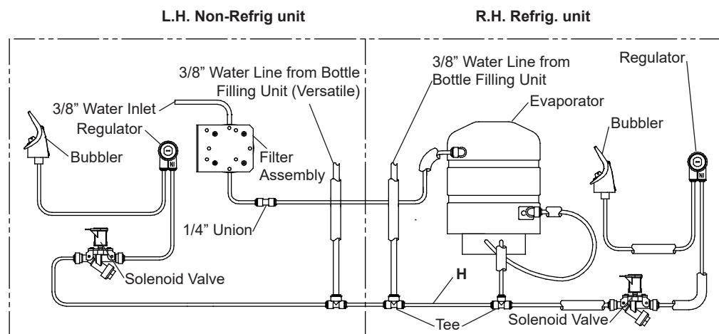
**EZ Bi-Level Plumbing Diagram after Filter Installation &
