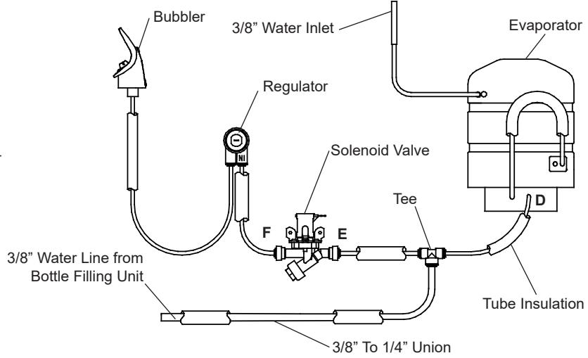
**EZ Plumbing Diagram after****Pressurization Modifications****Fig. 7B****L.H. Non-Refrig unit****R.H. Refrig. unit**
