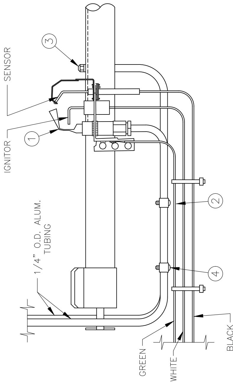
EP CONTROL SYSTEM - Q3452B PILOT ASSEMBLY
