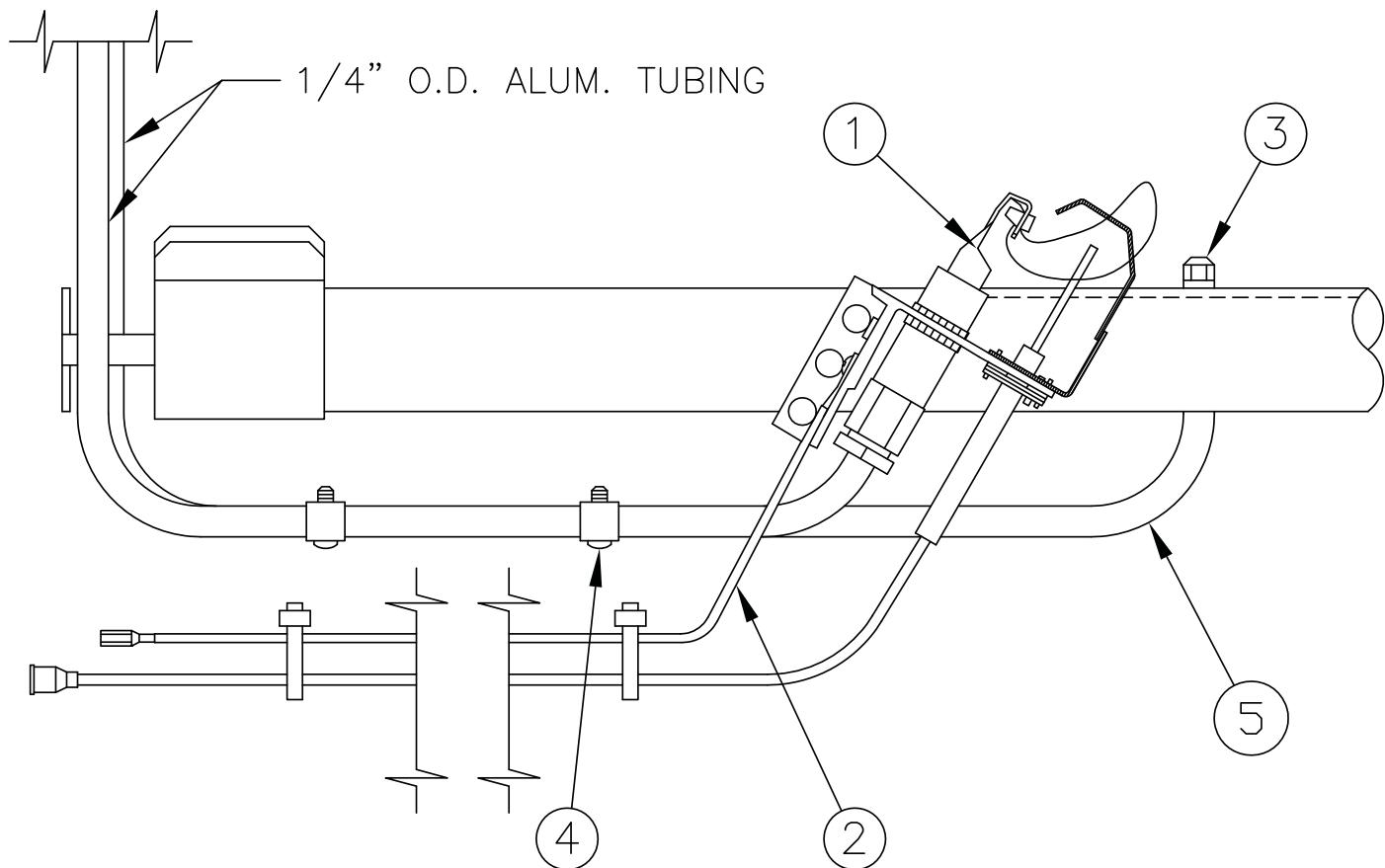
EI CONTROL SYSTEM - HONEYWELL Q3481 PILOT ASSEMBLY
