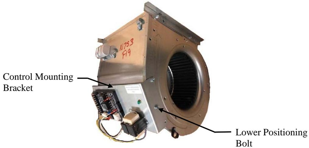
With the lower positioning bolt removed and the bracket rotated upward all of the connections are easily accessible for convenient installation and servicing as shown below.
