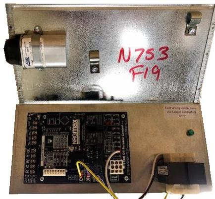
When finished with wiring and or servicing rotate the bracket to its original position and reinstall the lower positioning bolt.
