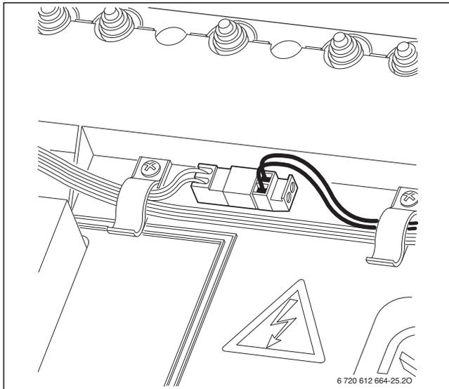
Fig. 49 Electrical wiring of external supply temperature sensor
