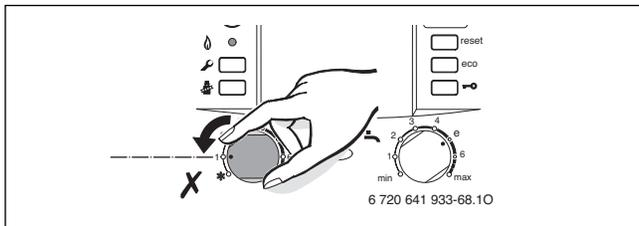
Fig. 68 Frost protection of the heating system
