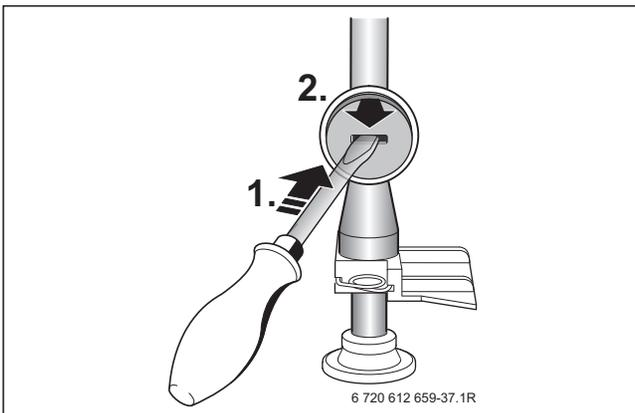
Fig. 78 Remove seal from the gas throttle
