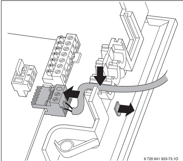
Fig. 45 Electrical connections DHW tank temperature sensor
