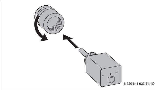
Fig. 24 Installing a LWCO device - LWCO adapter
