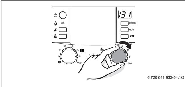
Fig. 65 Set the DHW temperature (heating boiler ZBR...-3A)
