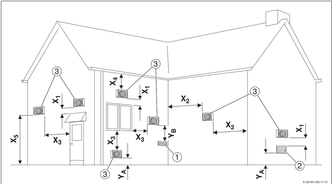
Fig. 31 Vent and combustion air pipe position
