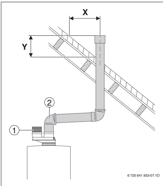
Fig. 37 Vertical venting system (room air only)
