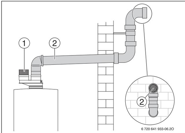
Fig. 32 Horizontal venting system (room air only)
