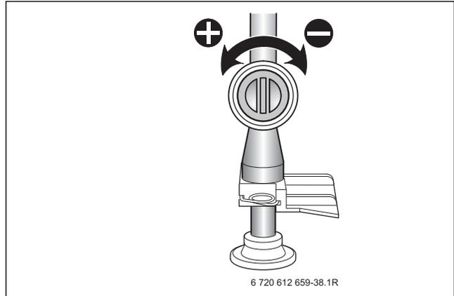
Fig. 79 Set CO<sub>2</sub> or O<sub>2</sub> level for maximum nominal output
