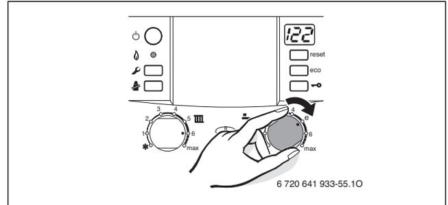
Fig. 66 Set the DHW temperature (combi boiler ZWB...-3A)
