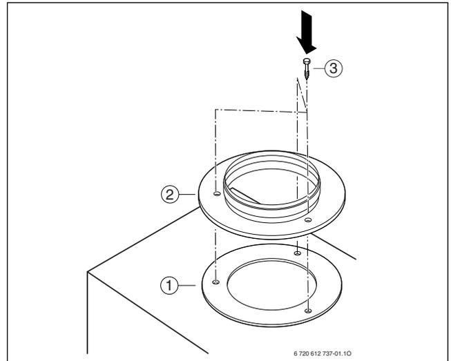
Fig. 26 Attaching the vent flange and gasket
