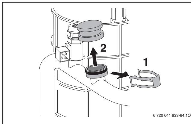
Fig. 23 Installing a LWCO device - removing dummy plug
