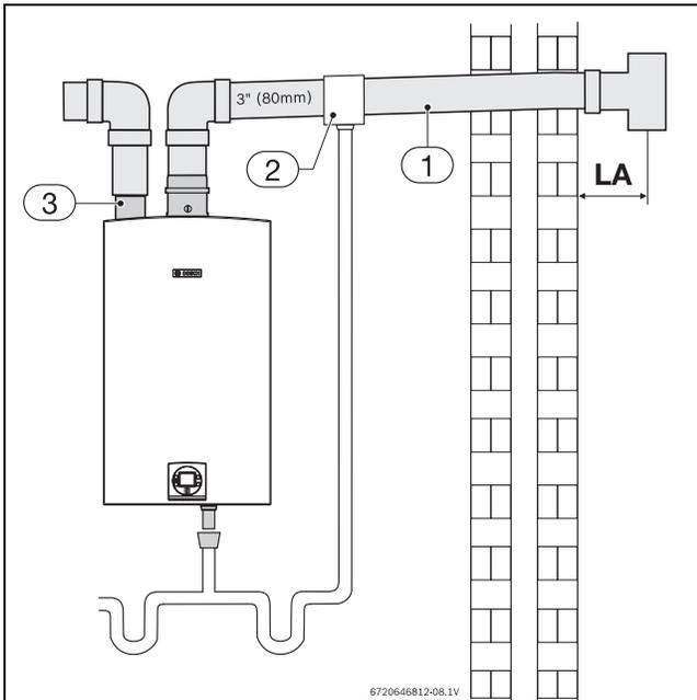
Fig. 15 Horizontal venting system (single pipe penetration)
