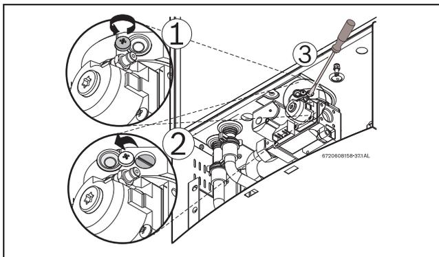
Fig. 69 Adjusting P1 CO<sub>2</sub> level
