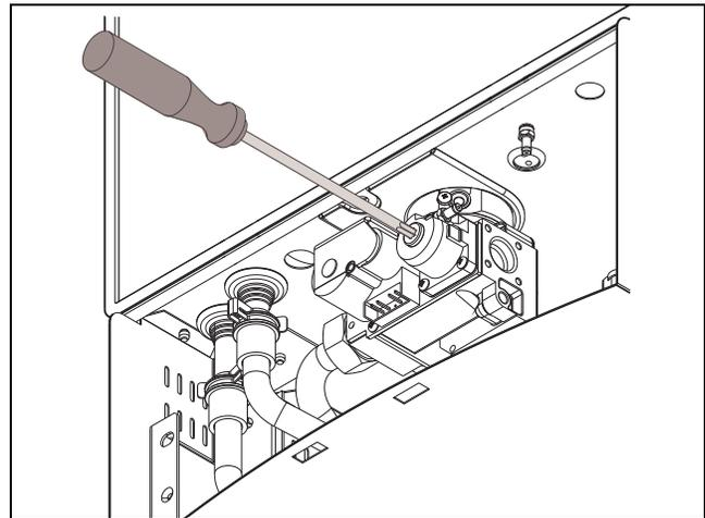
Fig. 70 Adjusting P2 CO<sub>2</sub> level
