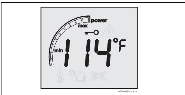
Fig. 63 Locked condition
