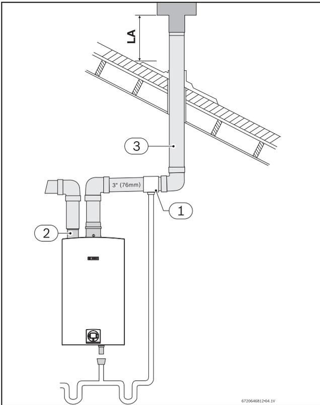
Fig. 11 Vertical venting system (single pipe penetration)
