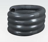
Are manufactured from polypropylene and feature rigid sections every 2' 3', and 4' Flex can be field cut and are ideal for use in chimneys with offsets. The base of your 3' and 4' Flex can be connected to InnoFlue® SW at any rigid section without coupler. Flex-to-Flex couplers available for extended flex runs.
