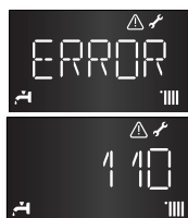
Figure 77 - Blocking Error Example
