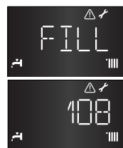
Figure 78 - Shut-Off Error for Low Water Pressure
