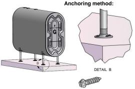
(16x) 1/4"dia. x 13/4" long Concrete Tapcon® Screws
