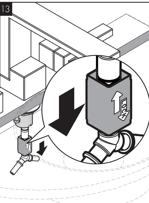
Lock the quick-connect by pulling down on it.
