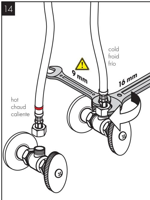
Connect the hot and cold supply hoses to the stops. Use two wrenches.
