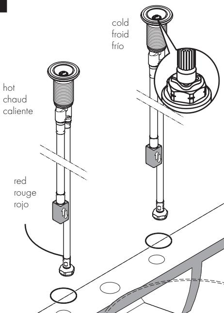
Place the hot and cold valve assemblies on the mounting surface.
