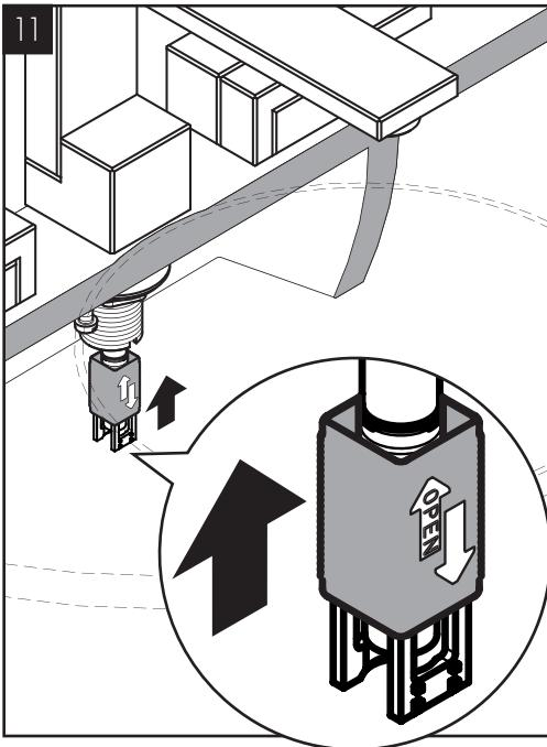
Open the quick-connect by pushing it upwards.
