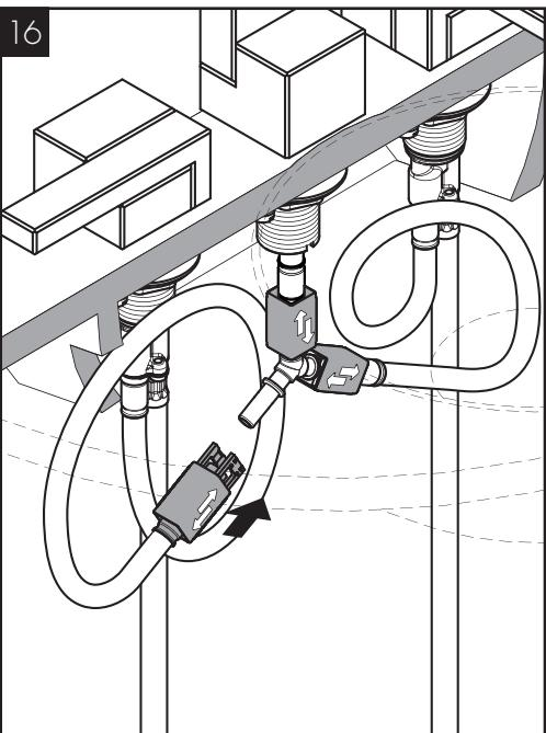
Push the quick-connect over one of the inlets on the connection angle.
