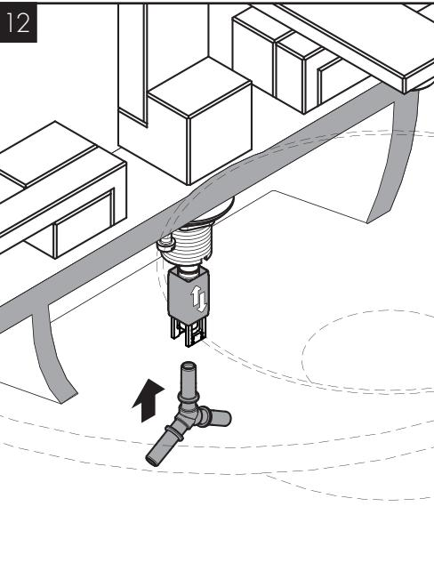
Insert the connection angle in the spout quick-connect.
