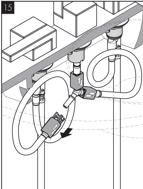
Open the quick-connect on one of the connection hoses by pushing it upwards.
