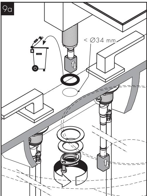
If the hole for the spout is less than  $1\frac{5}{16}$ " (34 mm), discard the 26x4 o-ring.
