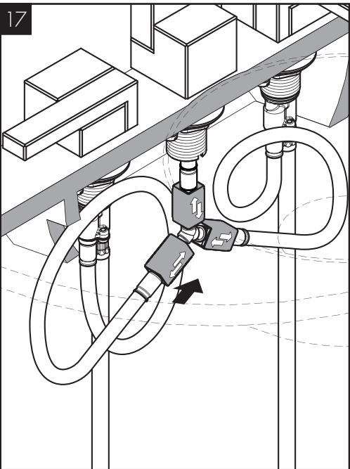
Lock the quick-connect by pushing it toward the connection angle.
