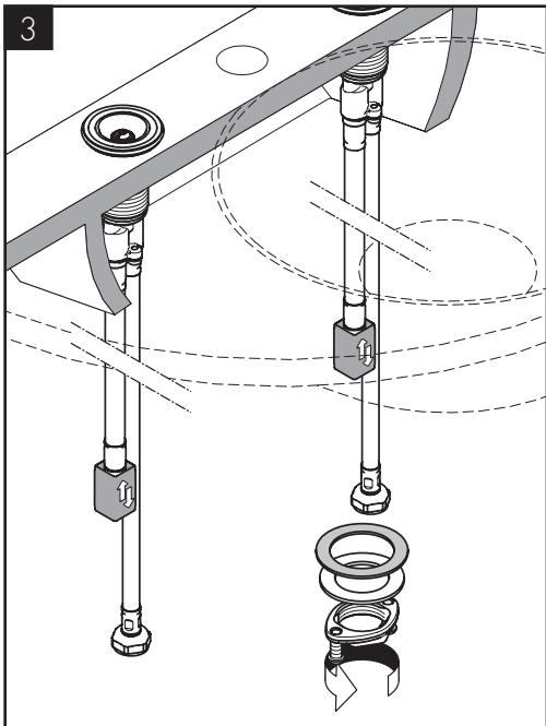
Install the fiber washer, metal washer, and mounting nut.
