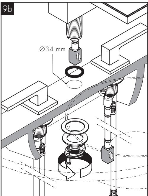
If the hole for the spout is  $1\frac{5}{16}$ " (34 mm), position the o-ring on the mounting surface.
