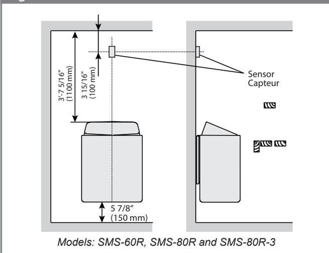
Figure 10 - Sensor's min. distance from an air vent
