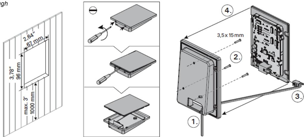
Figure 5 - Opening the Power Unit Cover and Mounting the Unit to a Wall
